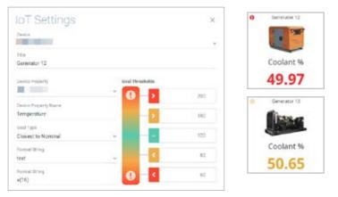
Indicators with thresholds set up for IoT widgets make it easy to spot the alerts.
