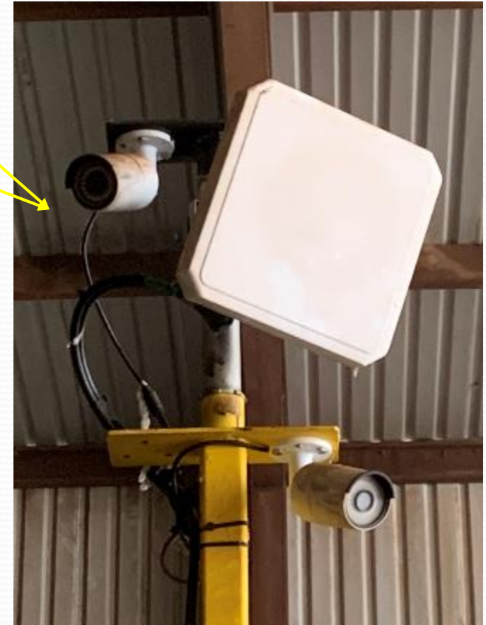
RFID Scanning Tower and IP Cameras to Record Unloading/Unwrapping Process
