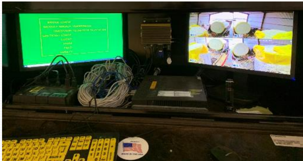
RFID Scanning System and NVR to Record Module Handling
