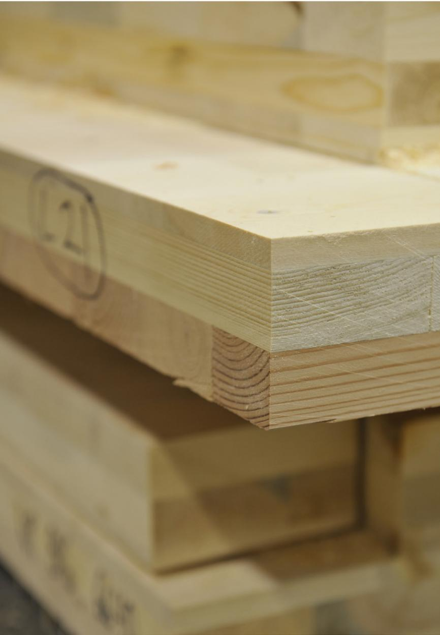
CLT is commonly used in post-and-beam and mass timber structures, as well as wooden bridges.
