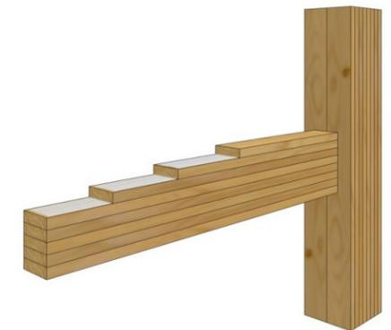
**GLT** is yet another form of glue-laminated timber that is used flat as panels for decking. Therefore, it is commonly used for floors and flat roof applications. It can also be used for elevator or stair shaft walls. It is typically produced in panels that are two feet wide and of different thicknesses. Currently, seven Canadian facilities produce GLT.
