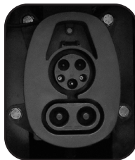
CCS "Combo" Charge Port (shown with dust covers removed)
