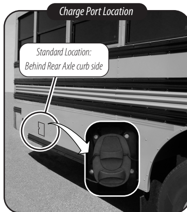
CCS "Combo" Charge Port (shown with dust covers removed)
