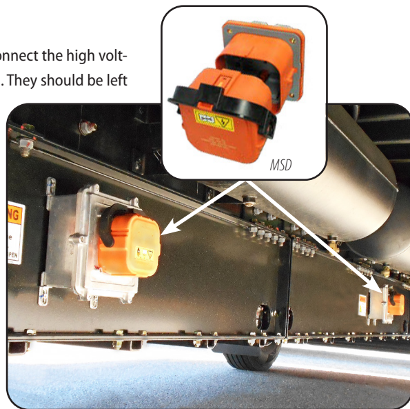
High Voltage Manual Service Disconnects (MSD) located on RH (Curb side) under skirt
