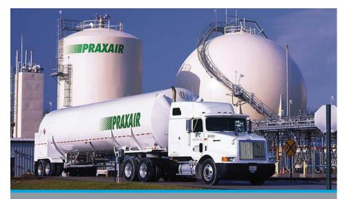
Gaseous hydrogen is liquefied by cooling it to below -253 °C (-423 °F). Once hydrogen is liquefied it can be stored at the liquefaction plant in large insulated tanks.
