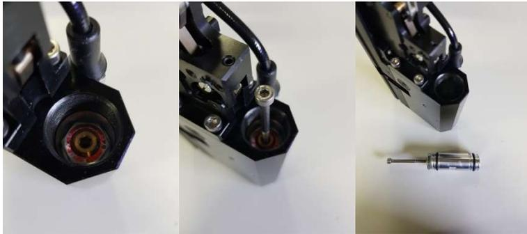
Wipe out the regulator chamber using a piece of paper towel. Now you can install the HuMa-Air regulator. Before installation apply a bit of silicone grease to the o-rings.
