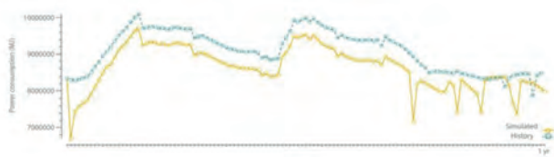
Figure 6. Calculated compressor power consumption (yellow) compared with historical data (green).
