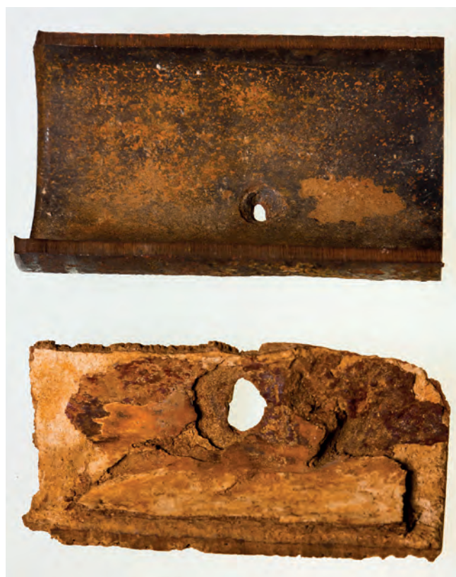
Figure 2. The presence of even small amounts of oxygen can increase the corrosion rate of steel and causes pitting and under-deposit corrosion, which pose a severe threat to the integrity of oil and gas pipelines.
