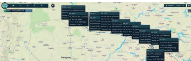
Figure 3. An example in Brazil of proposed flow and pressure set points recommended by simulation tools.
