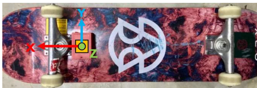
Figure 2 The placement of the instrumented device on the deck (rear view).
