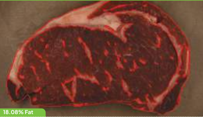
AI-enabled technology inspects color and calculates lean to fat content
