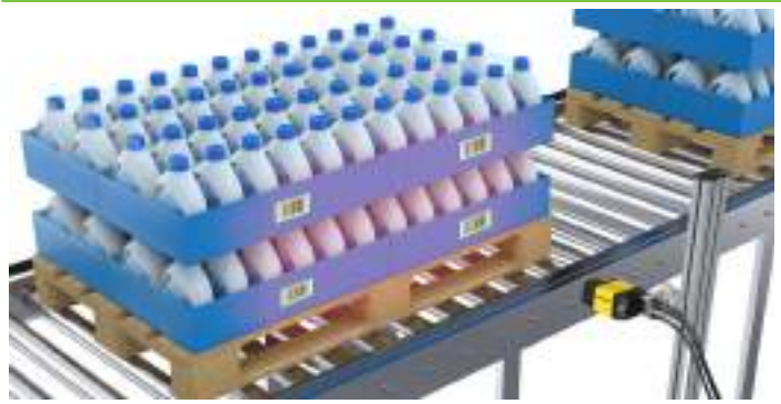
Barcode readers scan pallet labels on arrival
