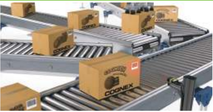
Barcode readers sort packages and track goods through a facility
