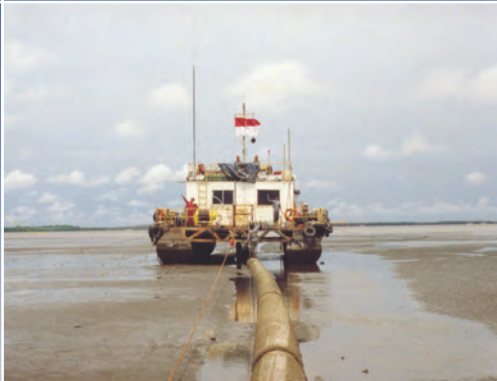
Inter Tidal trenching in mud flats 1.2 m to 20 meters (Lead Keel Machine)
