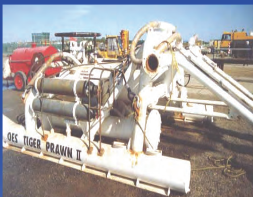
World's deepest water post trencher sled 1200 ft
