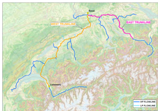
Figure 4. Schematic of a CO 2 collection network in Switzerland.
