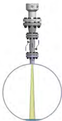
Figure 1. The process camera mounted on the gas pipeline.
