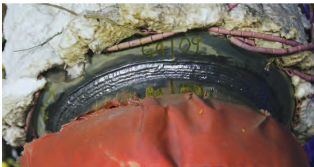
Figure 5. Circumferential weld made at test loop during simulated conditions.
