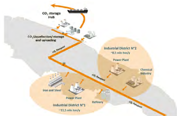
Figure 3. Schematic of a CO 2 collection network in southern Italy.
