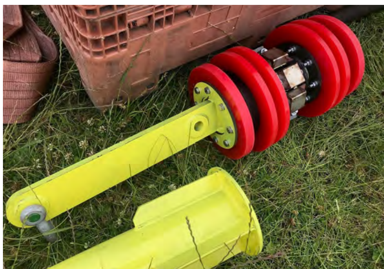
Figure 6. 12 in. cable pull-through pig.
