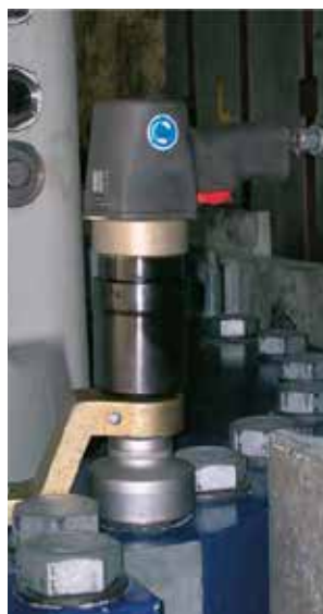
Alkitronic PC-S torque multipliers in use (figures on the right). Screw connections at a bolt circle and a diesel unit for large construction machines
