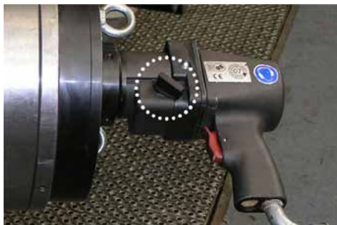
Alkitronic PC-F2, 2-gear pneumatic torque multiplier. Mechanically switchable from fast gear to power gear.
