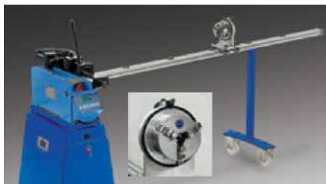
UNI 42 A, version with moving plane of bend and universal base (optional)
