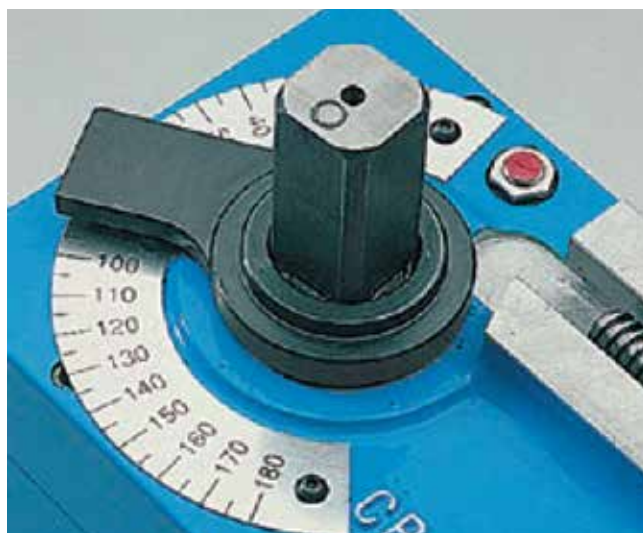
UNI 42 electric, with positioning ring to obtain the desired bending angle.
