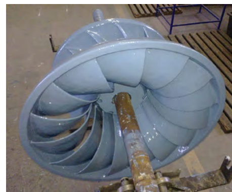
Efficiency improved on Francis turbine runner
