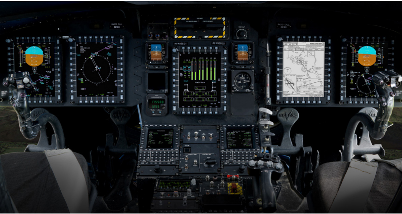
Collins has outfitted the CH-47F cockpit with its Common Avionics Architecture System (CAAS) to integrate multiple systems and optimize performance. (Photo courtesy of Collins)
