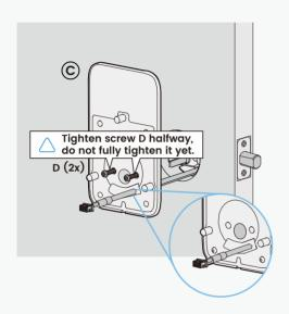
Push the cables through the notched gasket in the lower corner. Hold the mounting plate in place so its holes line up with the holes in the door. **Make sure the torque blade is in the center**. Turn the **D** screws in only halfway so the plate is not fully tight yet.
