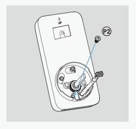
Tighten the cylinder screw clockwise with a screwdriver.
