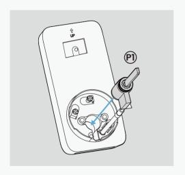
Insert the lock cylinder into the cylinder hole of the exterior assembly.
