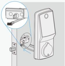
Place assembly and torque blade through the deadbolt slot and guide connection cables under the deadbolt as shown.
