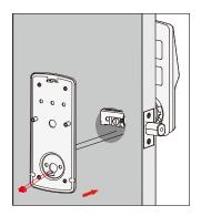
**2:** Align and secure mounting plate with adhesive strips. Guide connection cables through the hole and secure to the lower left notched hole.
