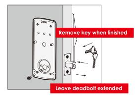
4: Use the key to ensure deadbolt locks and unlocks smoothly (no binding or rubbing). IMPORTANT: when finished, leave the deadbolt extended and remove the key before proceeding to the next step.
