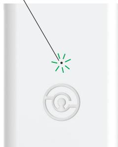
LED Indicator is located next to the Setup Button
