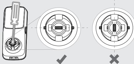
3. Using your fingers, press the two pins located on the left and right side of the lock to insert the handle back onto the lock.
