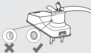
6. Rotate the key to horizontal and remove it.
