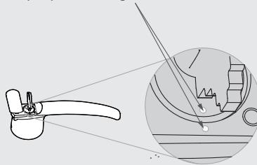
4. After confirming that the installation is complete, check whether the pin is popped up. Adjust the handle accordingly to ensure that the pins are fully released.
