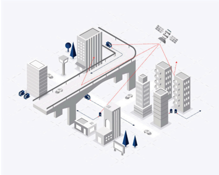
GNSS fails under bridges and near tall buildings
