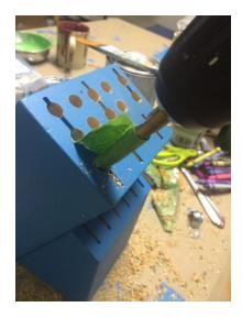
rules here other than try to keep the drill straight. Because of the knife slats, the wood can chip easily if you drill too fast. Go slow. Use the tape on the drill as a stop marker so you can keep the holes uniformly deep. I think 2" is about good.
