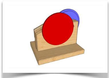
If you'd like a convenient way to store the sanding discs, you can drill 9/16" holes in the side of the Body opposite the Fence, and store the discs with the jig.
