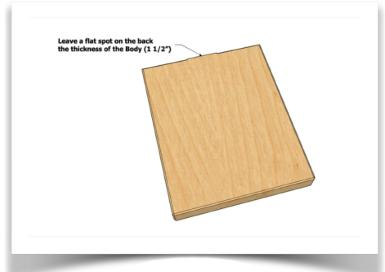
o Using a 1/4" round-over or chamfer bit in your router, or by sanding, ease all the edges of the Base, except leave a flat spot on the back edge of the Base the thickness of the Body (1 1/2").
