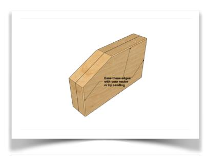
o Using a 1/4" round-over or chamfer bit in your router, or by sanding, ease the edges shown here of the Body.
