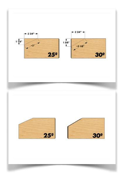
o Mark the Body block with these measurements according to the desired angle for your jig.
