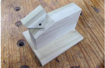
The attachment is the length of the ramp and ¾" thick by 1-3/4" wide with a ¼" wide groove down the center that holds the blade cut at the skew angle. To allow the attachment to be flipped and used on both sides of the ramp to sharpen right and left skew chisels, the center attachment hole is drilled half the thickness of the ramp away from the fence. A corresponding hole is drilled in the center of the ramp to accept the attachment.
