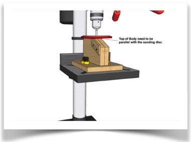
The jig will need to be calibrated to your drill press. Check to see that the edge of your chisels are ground to 90 degree. If not, calibrate jig to grind a perfect 90 degree edge on chisels by selectively applying blue tape to the bottom of one edge of the base.
