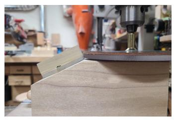
To sharpen the right skew chisel (see below), align the left-most side of the body (not including the attachment) with the center of the disc. Align the front edge of the attachment with the outermost edge of the disc (see above). Plunge the chisel into the disc in short 1-2 second bursts to sharpen.
