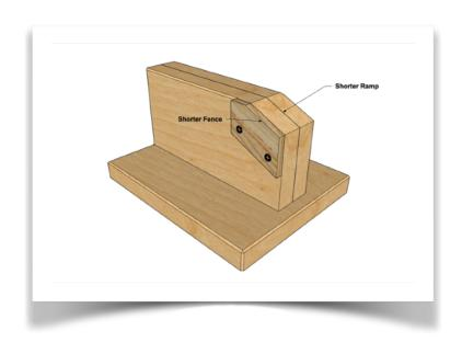
For chisels with shorter blades, make a jig with a shorter body. The example above has a body that is just 3" tall with a ramp that is at 25 degrees and just 1-3/4" long to accommodate a butt chisel with a 2-1/2" long blade.
