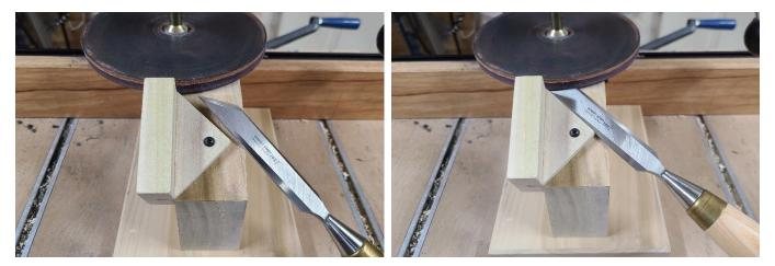
Hone the back and secondary bevel as described for standard bench chisels.
