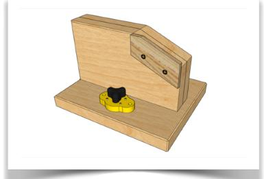
o Secure the Magswitch MagJig 95 Magnetic Clamps to the Base with the screws as per the instructions.
