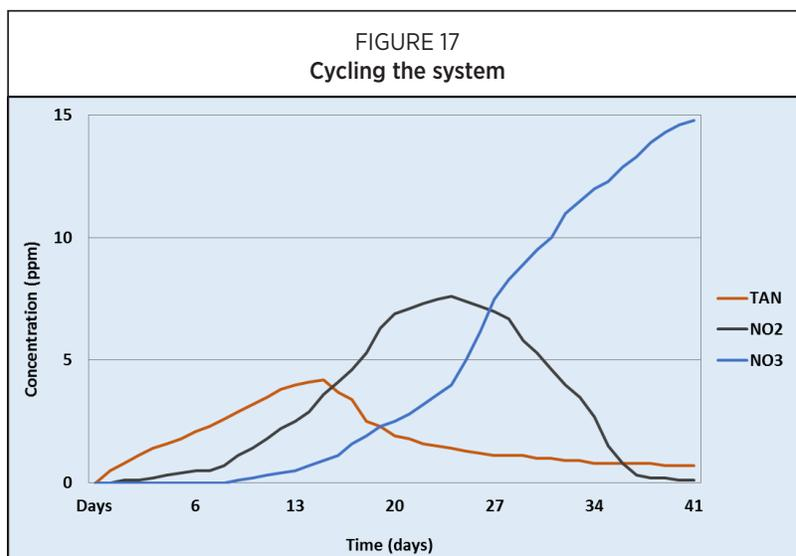
causes ammonia levels to spike, often resulting in fish death. Starting with 20% of the total fish capacity is a good rule of thumb. This allows the appropriate, system-specific biological organisms to colonize. If using a fish-less cycling strategy, household ammonia can be used. It is important to source surfactant-free ammonia, as it lacks detergents commonly added to these products that are unsuitable for the system.
