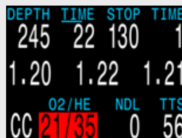
The CC diluent is red to indicate it is unsafe to breathe directly (PPO2 > 1.60)
