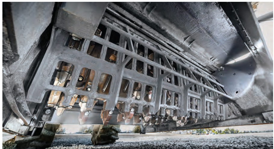
The vertically-stacked, hydraulically-adjustable classifying screens of the WRC 240(i) ensure that only material that has reached the desired grain size is output from the crushing process in the rotor housing.
