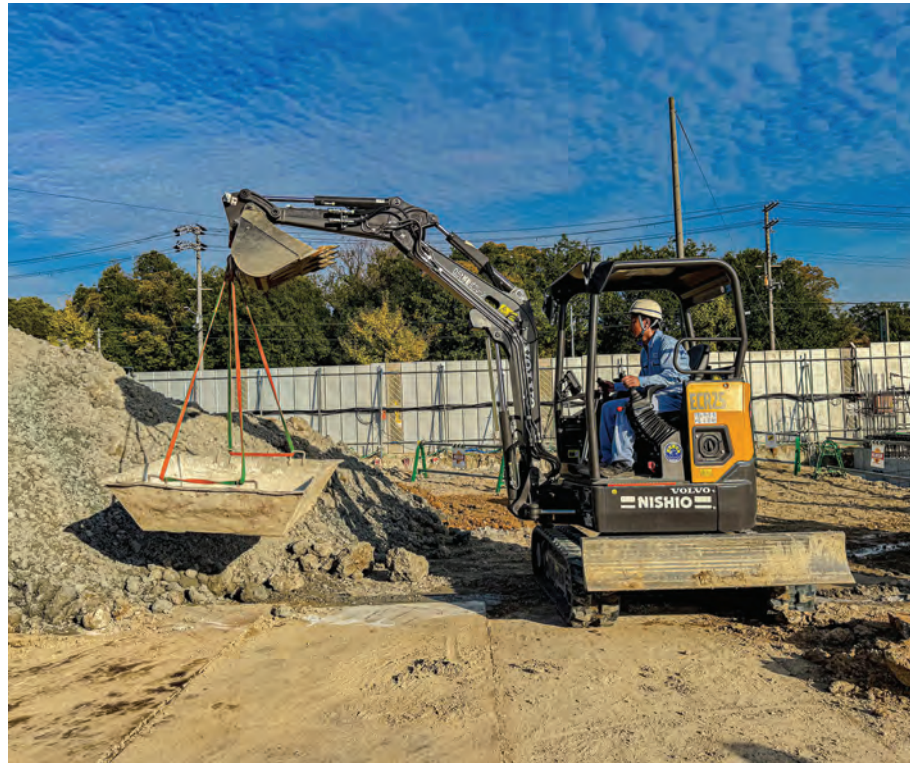
The Volvo ECR25 Electric compact excavator working on a residential project in Osaka. This 2.6-2.8 t capacity machine has an onboard charger for general charging, an external quick charger (optional for indoor/outdoor specifications), and a 20-kWh battery array, allowing for three to four hours of work per charge.
