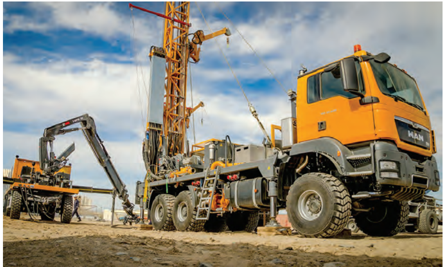
ABOVE: The new Bauer RB 65 mobile drilling rig features an electrical pilot control for a more economical and safer operation based on automation processes.
