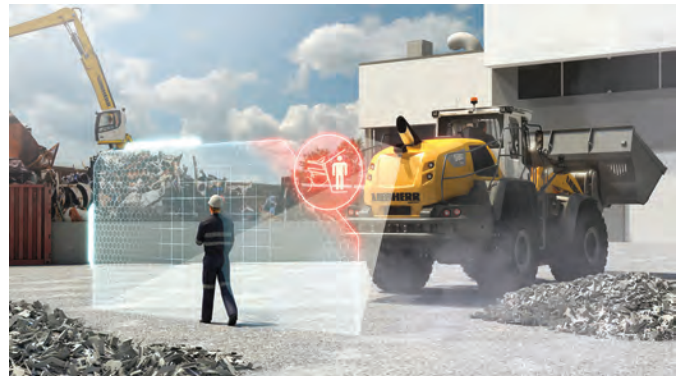
BELOW: For safety in wheel loader operation, active person recognition uses sensors and artificial intelligence to distinguish between people and objects.
