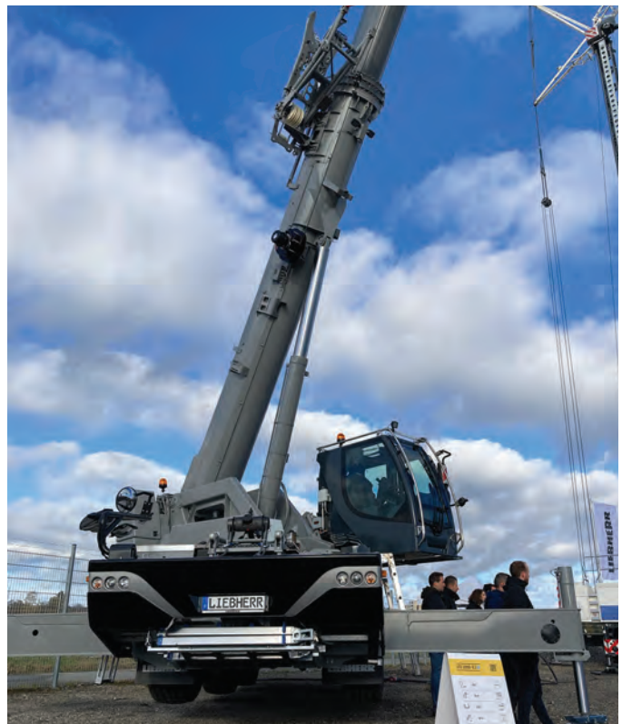
The LTC 1050-3.1 mobile crane can be powered by an electric motor, in addition to its six-cylinder engine.
