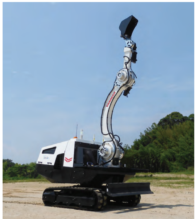
Yanmar's next-gen work machine prototype with force control technology, featuring zero emissions.
