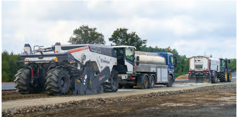
The Wirtgen WRC 240(i) rock crusher features a working width of 2,320 mm and a working depth of up to 510 mm, delivering an output of up to 600 t/hr.
