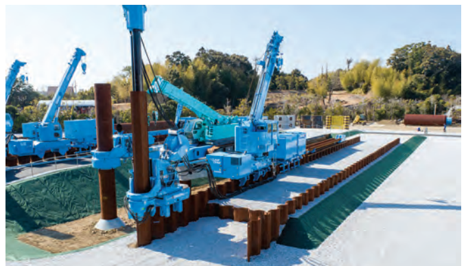
In the Demonstration Area, various construction sites are reproduced with real machines on an actual scale, such as the Silent Piler and GRB System.
