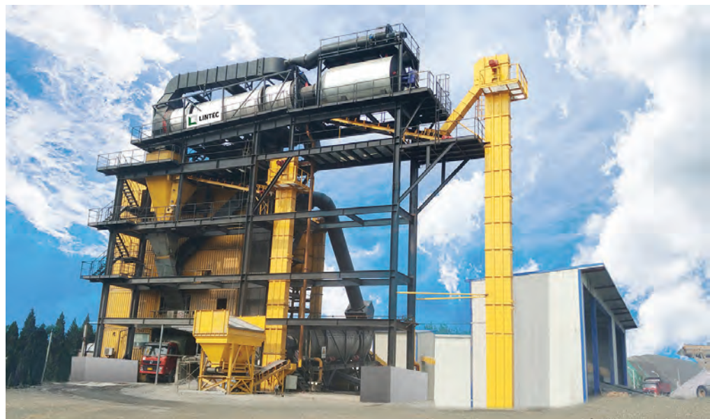
A Lintec asphalt plant in operation in China. This unit is fitted with a hot recycling system that delivers a number of environmental benefits, and also features the containerised concept for easy transportation.
