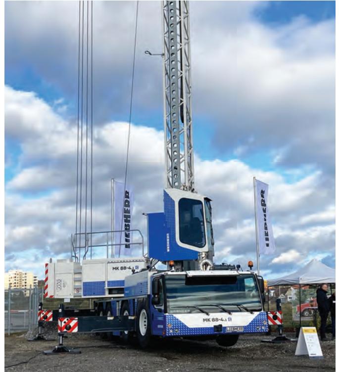
The MK 88-4.1 mobile construction crane features a hybrid power concept.
