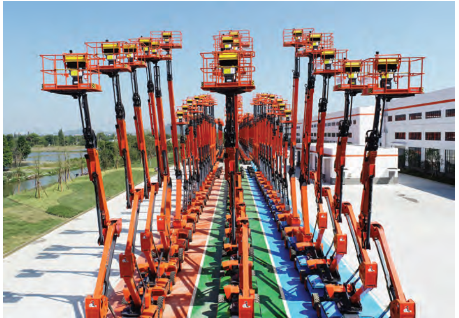
ABOVE AND BOTTOM: Dingli's large-capacity boom lifts with a modular design include the D-, M- and T-series, covering working heights from 16 to 44 m. They offer three types of power sources: diesel (orange), electric (green) and hybrid (blue).
