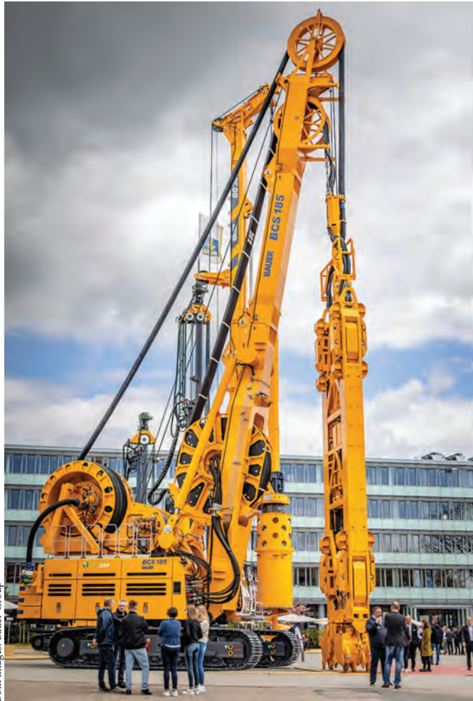
LEFT: The new Bauer BCS 185 cutter system can cut trenches up to a depth of 90 m. One of its highlights is the turnable HDS 90-T hose drum system.
