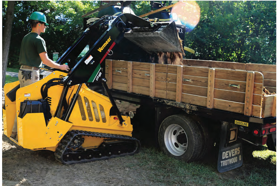
The CTX100 mini skid steer has a tipping capacity of 1,334 kg and a rated operating capacity of 467 kg. Vermeer has also increased the hinge pin height to 227.33 cm to make loading materials into a brush chipper, truck or trailer more efficient.
