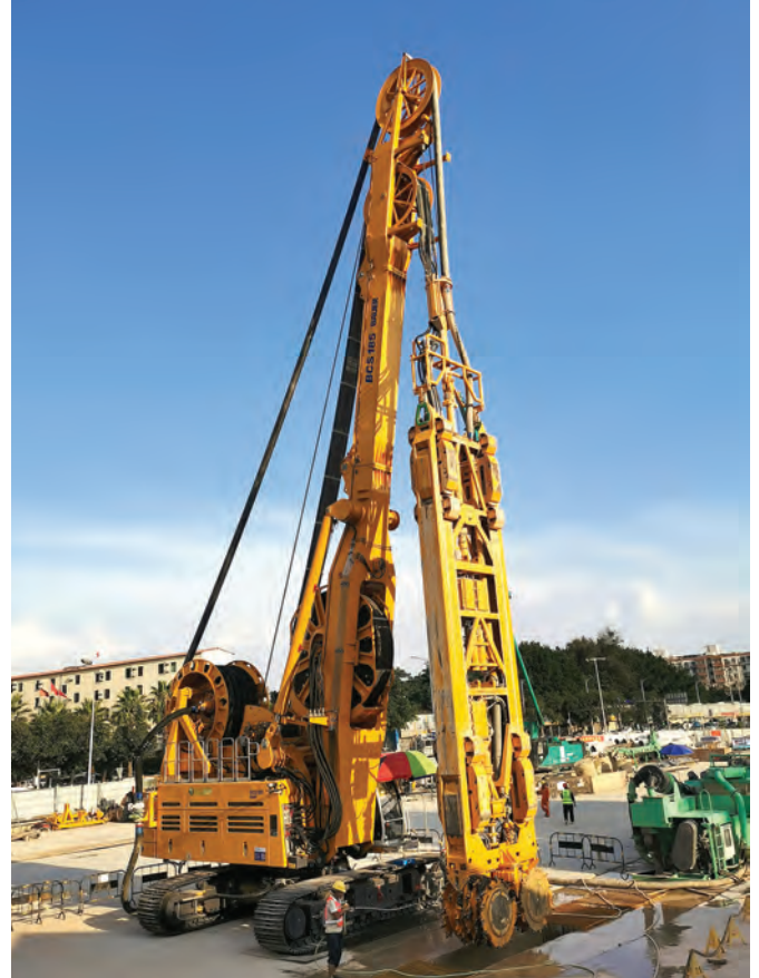
LEFT: The new Bauer BCS 185 cutter system can cut trenches up to a depth of 90 m. One of its highlights is the turnable HDS 90-T hose drum system.
