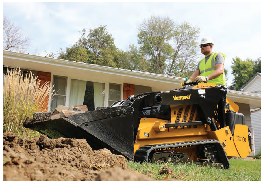
The CTX160 mini skid steer offers a rated operating capacity of 725 kg, 56.8 l/min of auxiliary hydraulic flow and a width of 106.7 cm. The machine delivers all-around performance while remaining compact and nimble to operate.
