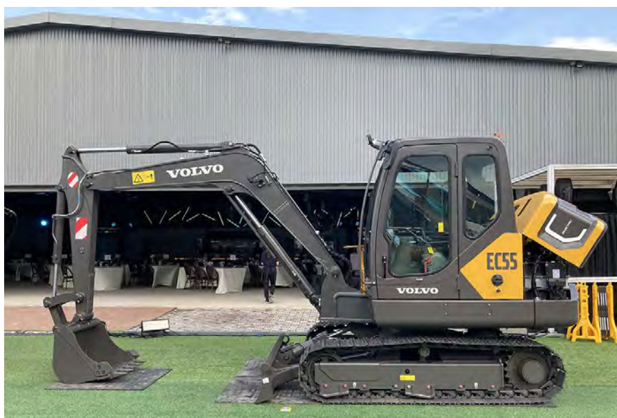
The new electric machines introduced by Volvo CE to the Southeast Asian market include (from top) the L25 Electric compact wheel loader, ECR25 Electric compact excavator and EC55 Electric excavator. All of them are battery-powered, and offer the same productivity benefits as their diesel equivalents.
