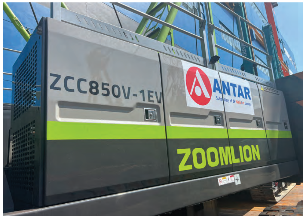
TOP AND ABOVE: The Zoomlion ZCC850V-1EV has a boom length of 13-61 m, fixed jib length of 7-19 m, maximum lifting capacity of 85 t and maximum lifting moment of 363 tm. The travelling speed is up to 1.4 km/hr, with a gradeability of 30%.
