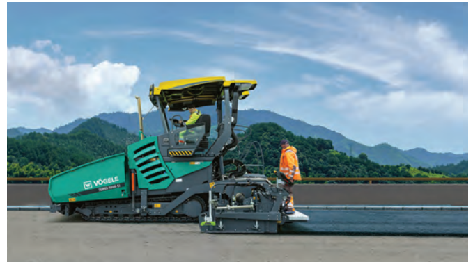
The new Vögele Super 1800-5(i) paver with the latest 'Dash 5' technology is ideal for pave widths of between 2.55 and 10 m.
