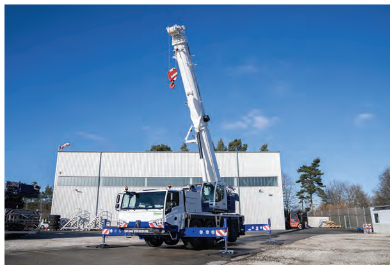
TOP AND ABOVE: Tadano's new hybrid all-terrain cranes feature a battery electric superstructure. One of the models, the 70-t AC 4.070HL-1 (pictured), is now available to the market.
