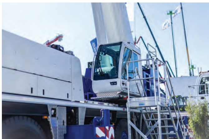
ABOVE AND BELOW: The 120-t Tadano AC 5.120H-1 hybrid all-terrain crane is the latest model in the series.
