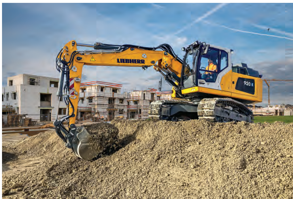
The R 920 G8-E is the first battery-powered electric crawler excavator developed by the Liebherr Group.
