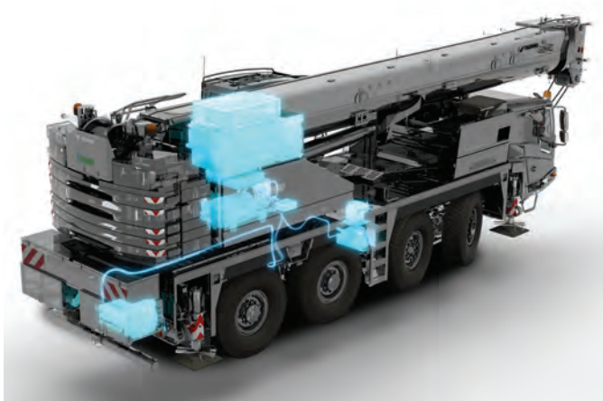
TOP AND ABOVE: A combination of conventional travel and fully electric on-site operation is made possible by using the new hybrid cranes. The units can be operated both self-sufficiently with their own battery power and with the support of an external power source.
