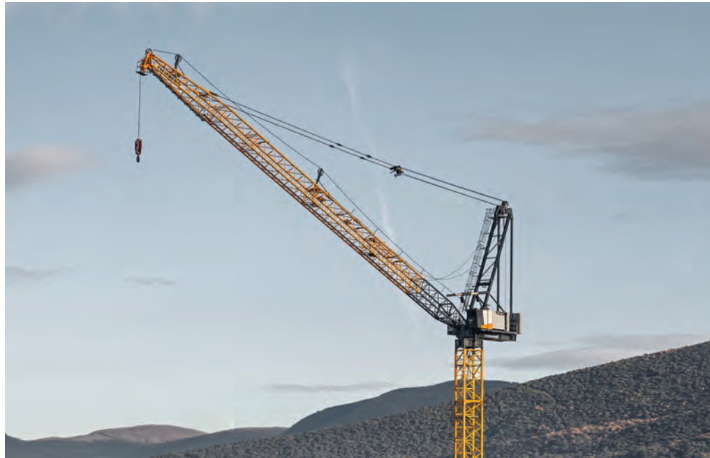
The new 620 HC-L offers an out-of-service position of 12 m and a minimal operating position of just 4.1 m.
