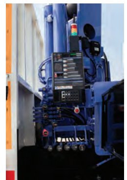
BELOW: AML with Safety Eyes provides a greater degree of vision and control for the operator. It monitors overload momentum during work and warning/stops once momentum is reached 100%.
