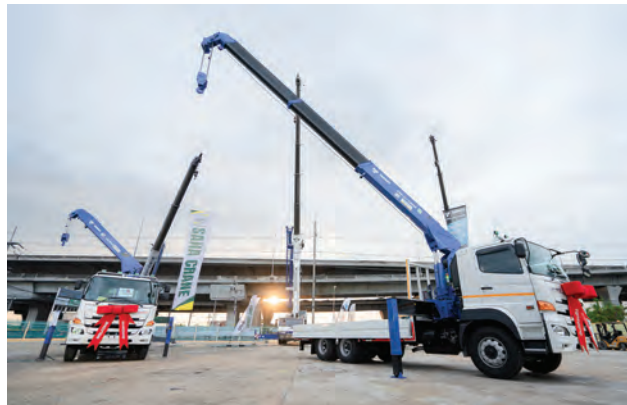
LEFT AND BELOW LEFT: The new Tadano TM-ZX1205HRS loader crane features a maximum lifting capacity of 12 t and maximum outrigger width of 5.5 m.
