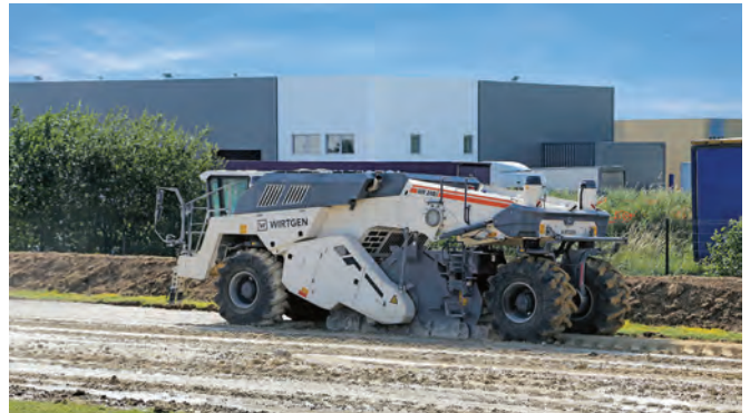
ABOVE AND LEFT: The new AutoTrac automatic steering system makes Wirtgen cold recyclers and soil stabilisers more efficient.
