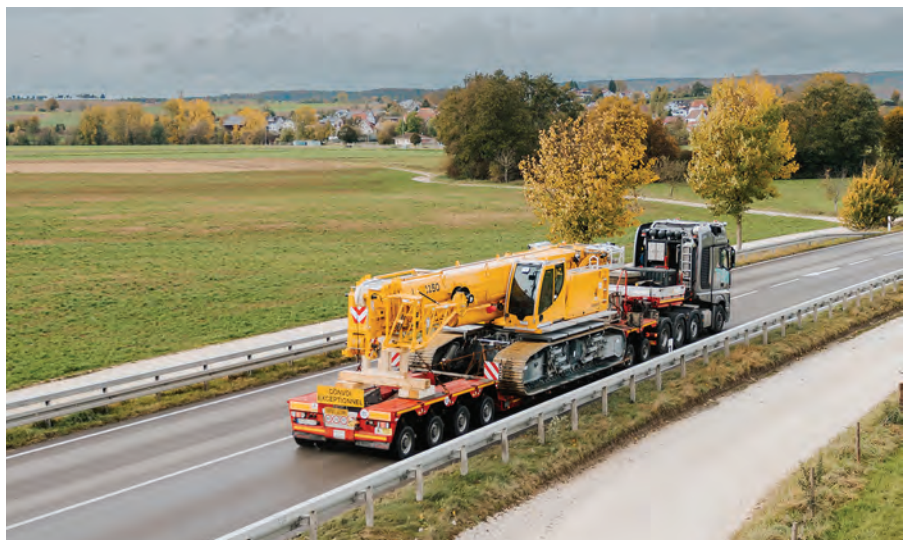
BELOW: The LTR 1150 can be transported complete with crawler carriers on a low-loader with a total weight of only 60 t and a width of 3.5 m.
