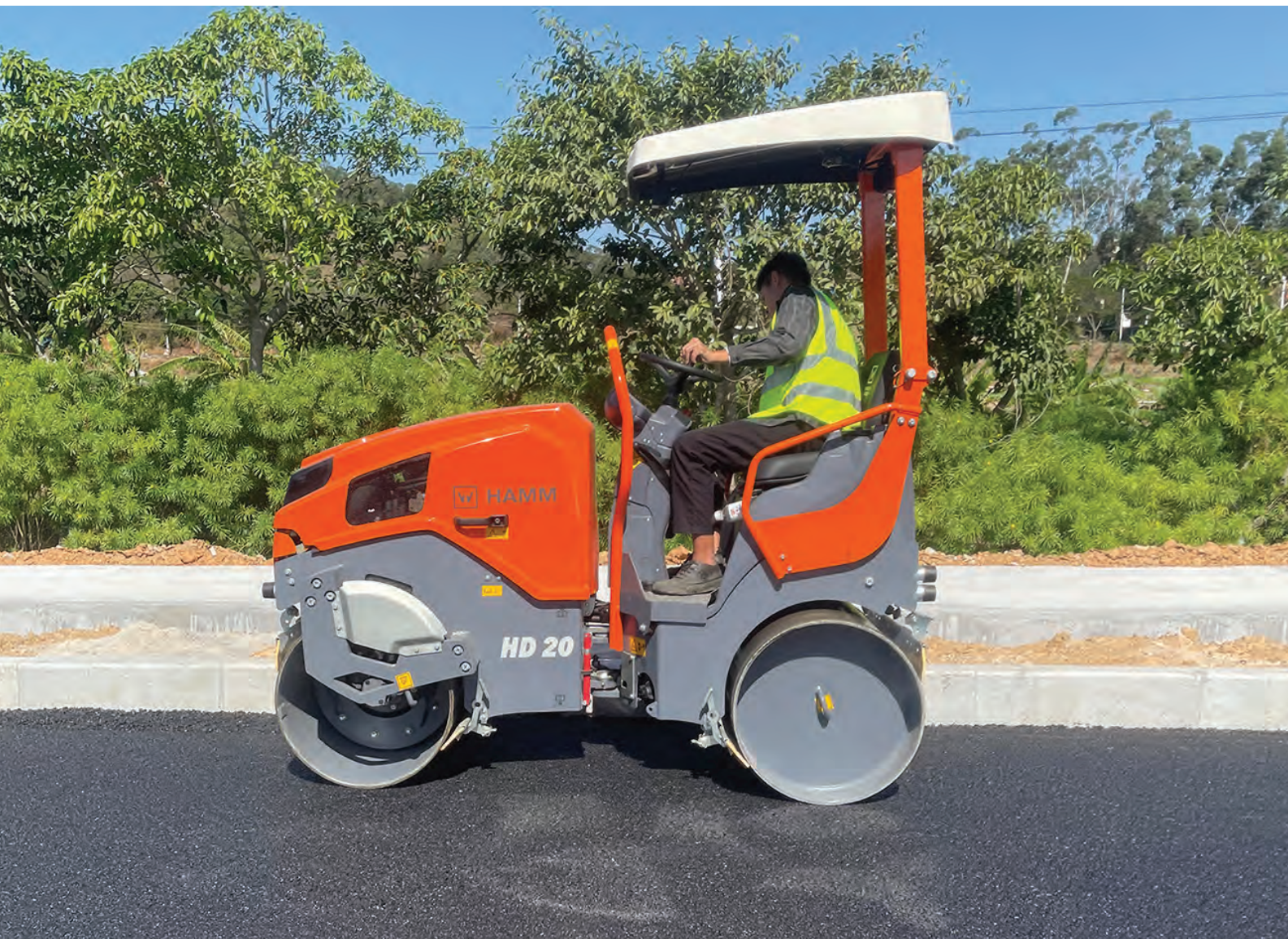
The HD 18 and HD 20 rollers have operating weights of between 1,590 and 1,680 kg, making them ideal for small jobsites.
