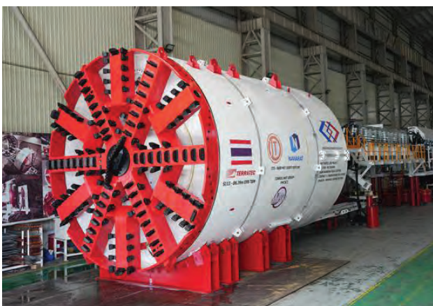
Terratec TBMs feature the Enzan laser guidance system, which allows for remote access to the complete tunnelling system, thus ensuring accurate control over the TBM operations.
