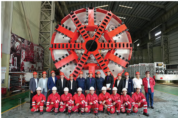
Two new Terratec EPB TBMs will take part in the Bangkok Metro Purple Line (C3) project in Thailand. The machines will be used to build a total tunnel length of 3.12 km.
