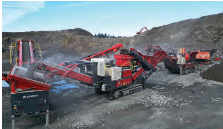
ABOVE AND LEFT: The new QH443E is Sandvik's flagship Q-Range electric-driven cone plant. The unit is ideal for secondary or tertiary crushing in aggregate production, quarries and mines.
