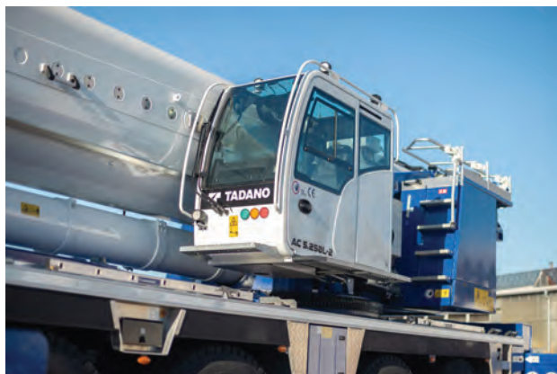
TOP, ABOVE AND LEFT: Tadano will unveil its new AC 5.250L-2 all-terrain crane at bauma. This latest model is equipped with a main boom length of 79 m.
