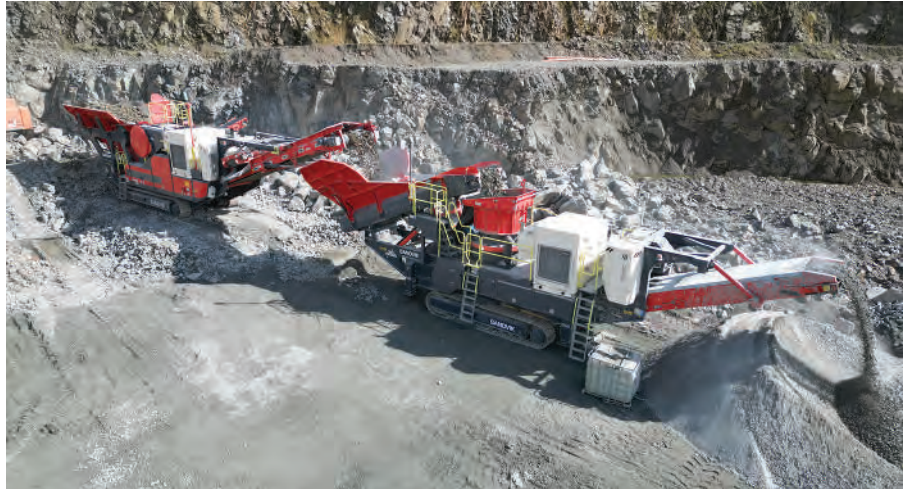
ABOVE AND LEFT: The new QH443E is Sandvik's flagship Q-Range electric-driven cone plant. The unit is ideal for secondary or tertiary crushing in aggregate production, quarries and mines.
