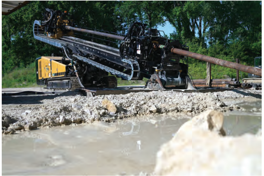
The use of AutoTension optimises reamer penetration through consistent tension application and improves positioning and control of the reamer within the bore hole.
