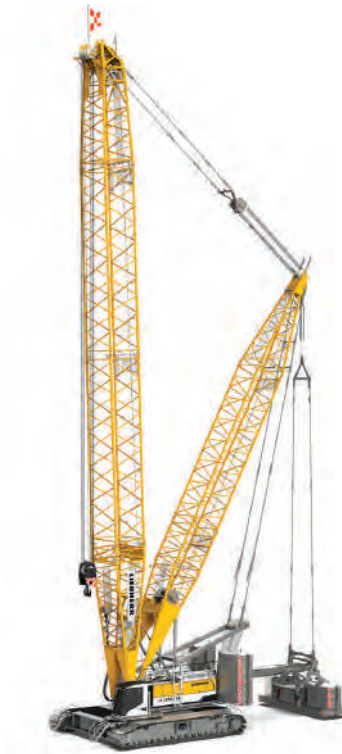
LEFT: At bauma, Liebherr will unveil a battery-powered unplugged version of the 300-t LR 1300 SX crawler crane.
