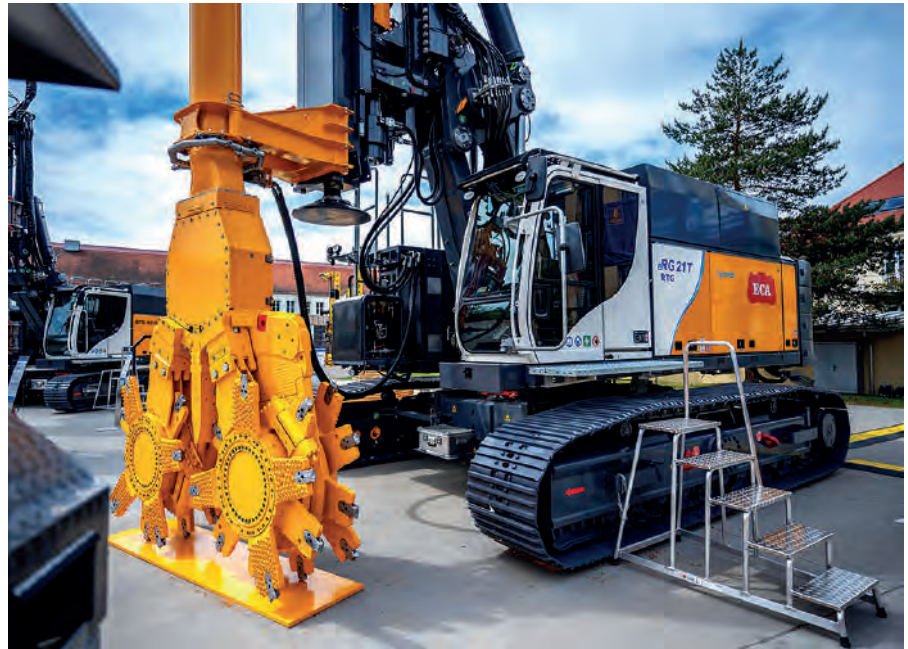
Hybrid operation of the eRG 21 T hybrid reduces fuel consumption, and thereby also CO 2 emissions, by up to 68%.
