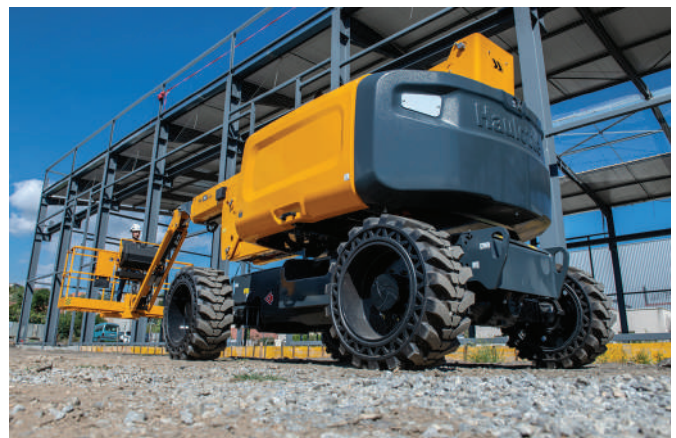
The automatic differential lock provides extra traction on uneven or sloppy ground, allowing the operator to maintain full manoeuvrability and navigate obstacles without difficulty.
