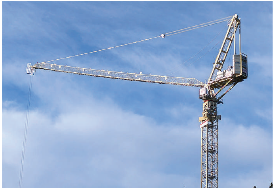
The new Jaso J638PA luffing crane features a maximum reach of 65 m, with a maximum load capacity of 32 t and a maximum tip load of 7.2 t at its full reach.
