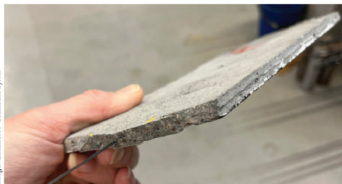
Concrete with embedded carbon fibre textile.
