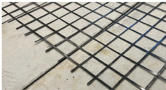
Carbon fibre textile reinforcement mesh.
