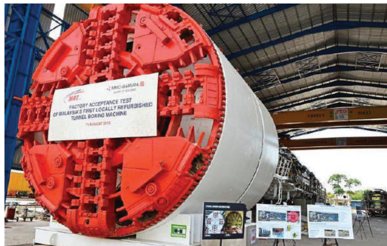
The A-TBM in Malaysia. This autonomous TBM has been developed in-house by Gamuda.
