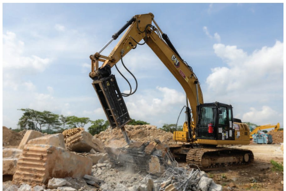
BELOW: Large-diameter hammer tools feature high frequency and impact power to quickly break through tough rock and concrete.
