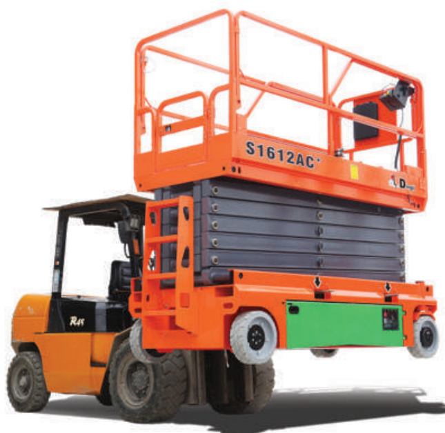
ABOVE: The new Dingli AC+ scissor lift series covers working heights from 8 to 16 m and capacities from 250 to 350 kg.
