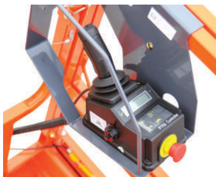
ABOVE: The platform's new control box has a larger display screen.
