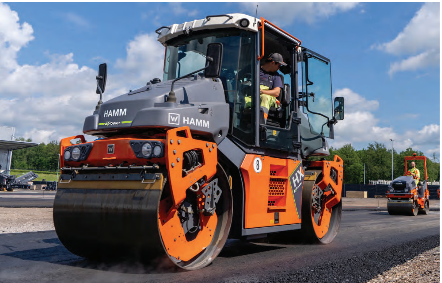
ABOVE AND LEFT: The Hamm HX 70e electric tandem rollers are powered by a 400-V battery with a capacity of 63 kWh. Using the fast charge option, the battery can be charged from 20% to 80% in under an hour.
