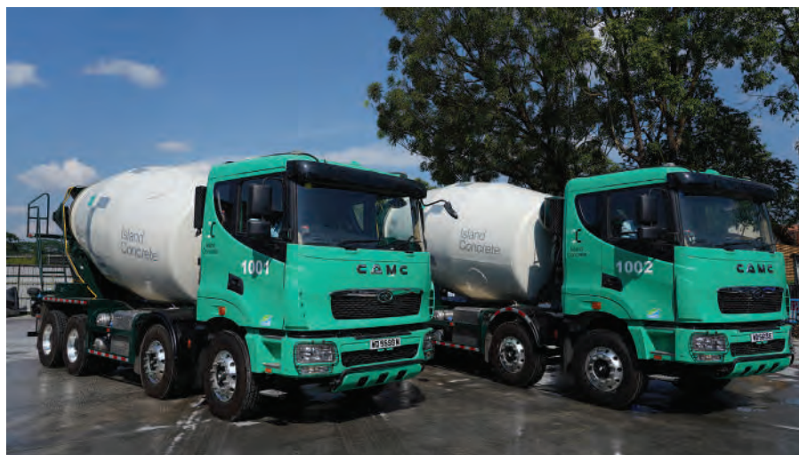
The use of 12 cu m concrete mixer trucks also allows site casting to be completed much faster with shorter waiting times. As a result, construction projects can be delivered earlier.
