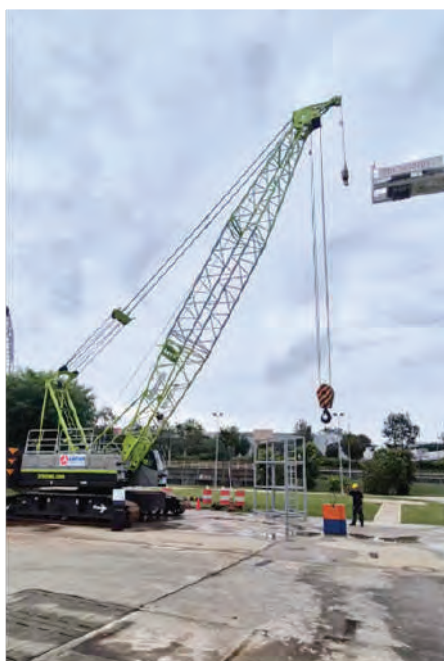
The ZCC850V-1EV electric crawler crane is powered by a 166.3-kWh battery pack, which is capable of running for about eight hours or more when fully charged, depending on the application.
