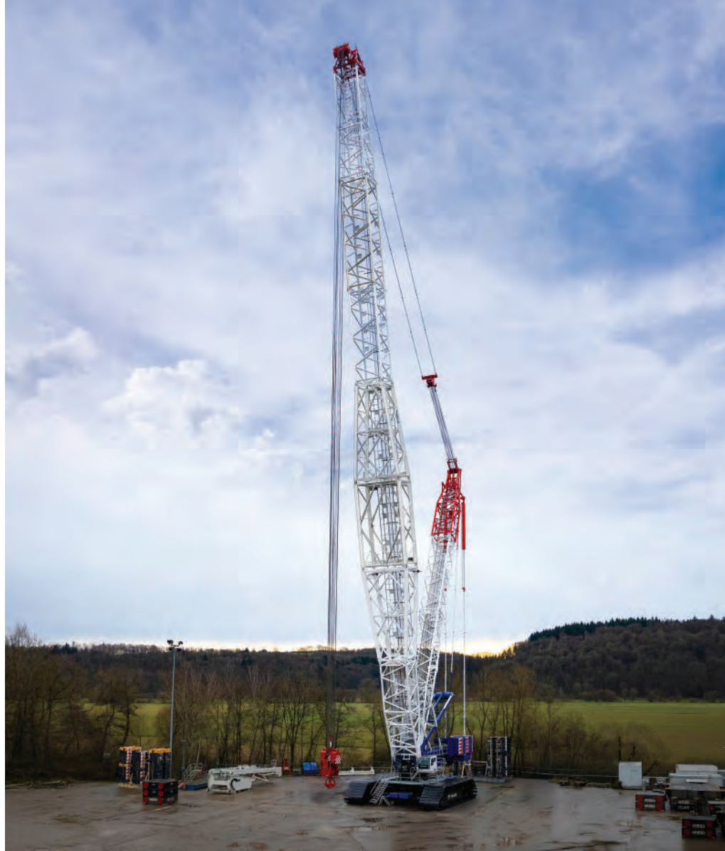
For jobsites with uneven terrain, an optional Pedestal Crane (PC) kit replaces the crawlers on the undercarriage with outriggers, enabling precise levelling at three different outrigger bases. In addition, the crane’s engines are compatible with HVO fuel, reducing CO2 emissions without sacrificing performance.
