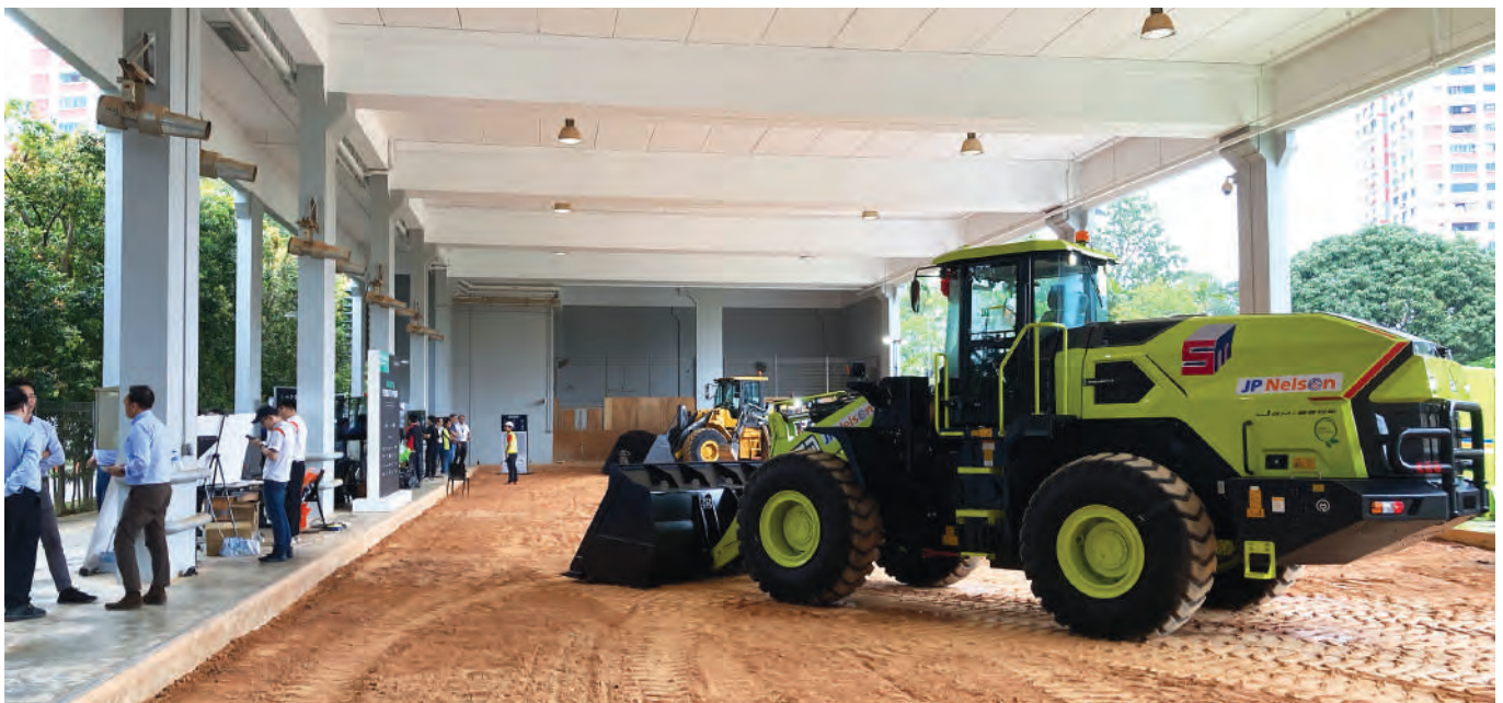
JP Nelson's electric crawler crane (above) and electric wheel loader (below) are suitable for use in urban areas, especially in projects with high environmental protection requirements.
