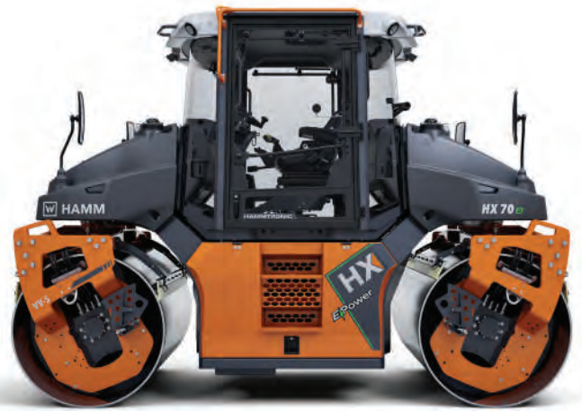
ABOVE AND LEFT: The Hamm HX 70e electric tandem rollers are powered by a 400-V battery with a capacity of 63 kWh. Using the fast charge option, the battery can be charged from 20% to 80% in under an hour.
