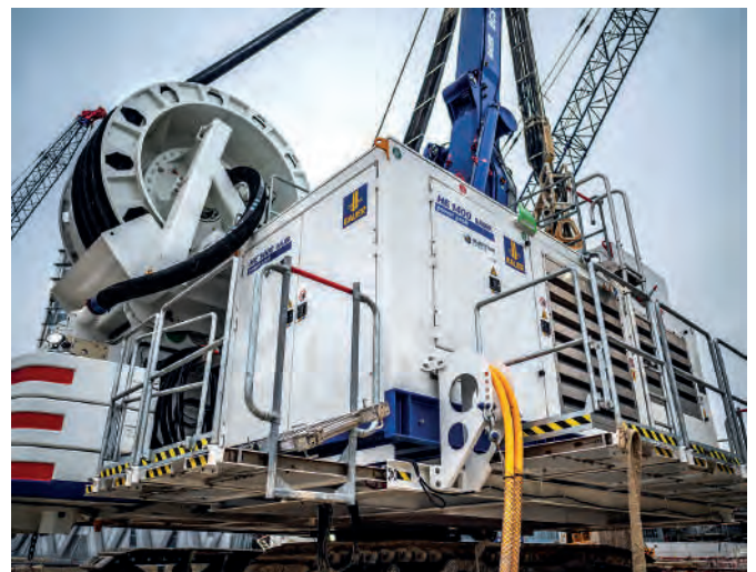
TOP AND ABOVE: The new Bauer BCS 185 power pack features a modular drive concept, allowing operators to choose between an electric motor and a diesel unit.
