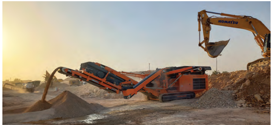
ABOVE: The R1100DS crusher features Rockster's Duplex System, which enables interchangeable crushing units on one basic machine.
