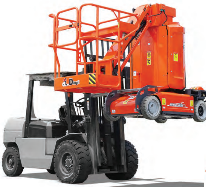
The new vertical mast has special fork loading holes to enable easy transport.
