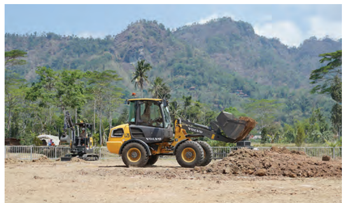
ABOVE: The Volvo L25 Electric compact wheel loader has a 40 kWh battery pack.
