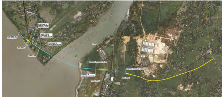
Passing 20 m under the Karnaphuli river, reaching 31 m deep, the Bangabandhu Sheikh Mujibur Rahman Tunnel is touted as the first slurry shield under-river road tunnel in South Asia. SMEC was appointed to undertake design review, contract management and construction supervision for the project.
