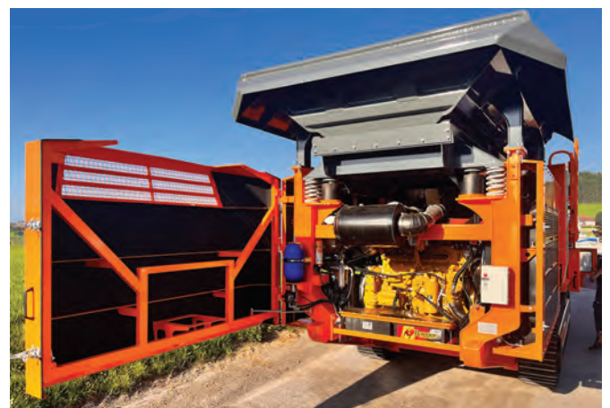
ABOVE: For simple service and maintenance, the R1100DS has large engine bay openings that allow easy access to the inner workings of the crusher.
