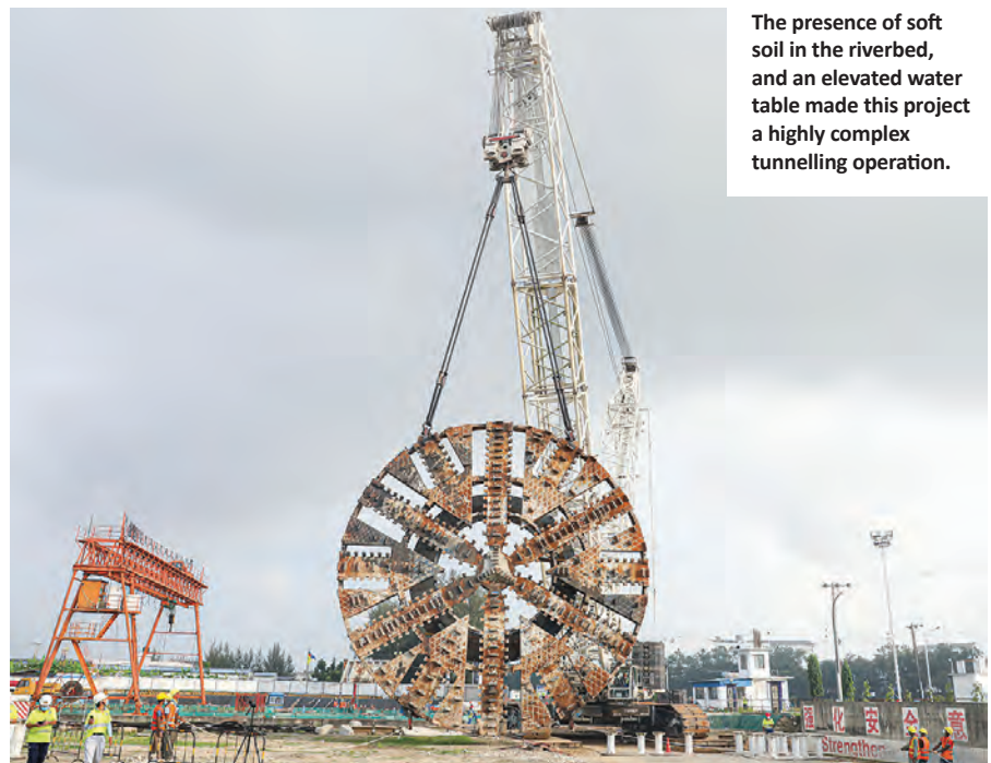
Passing 20 m under the Karnaphuli river, reaching 31 m deep, the Bangabandhu Sheikh Mujibur Rahman Tunnel is touted as the first slurry shield under-river road tunnel in South Asia. SMEC was appointed to undertake design review, contract management and construction supervision for the project.
