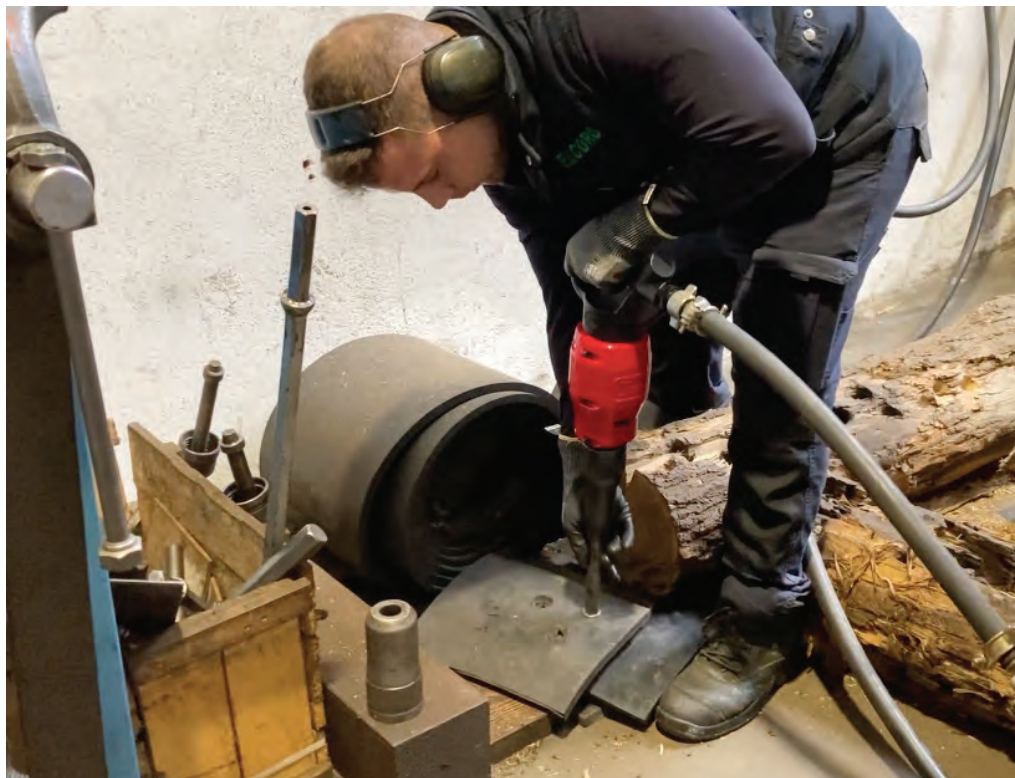
ABOVE: Topac demonstrated the capabilities of its hammers during the press event. These hammers feature a functional and ergonomic design, with a reduced number of parts and an air chamber system.
