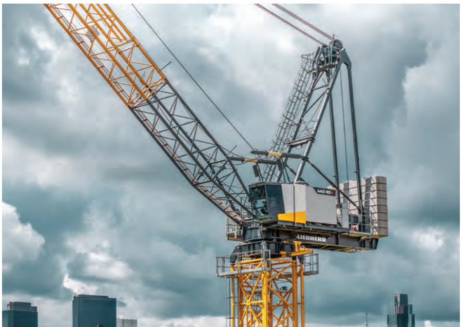
This new luffing jib crane has an out-of-service position of less than 11 m.
