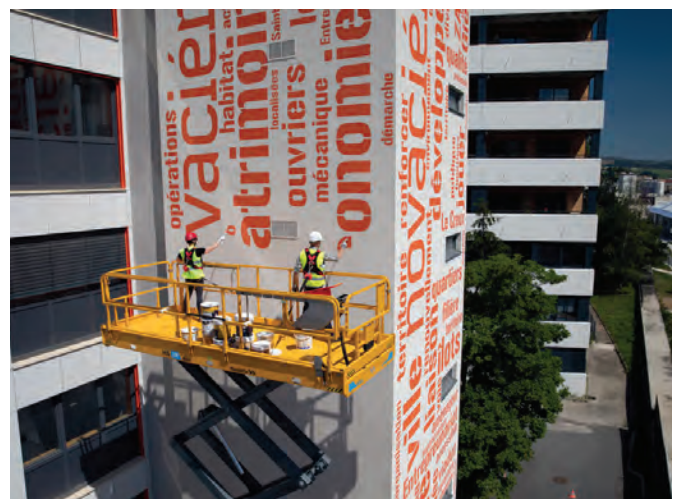
The HS18 E MAX scissor lift can drive at full height (with a full load), reaching up to 18 m.
