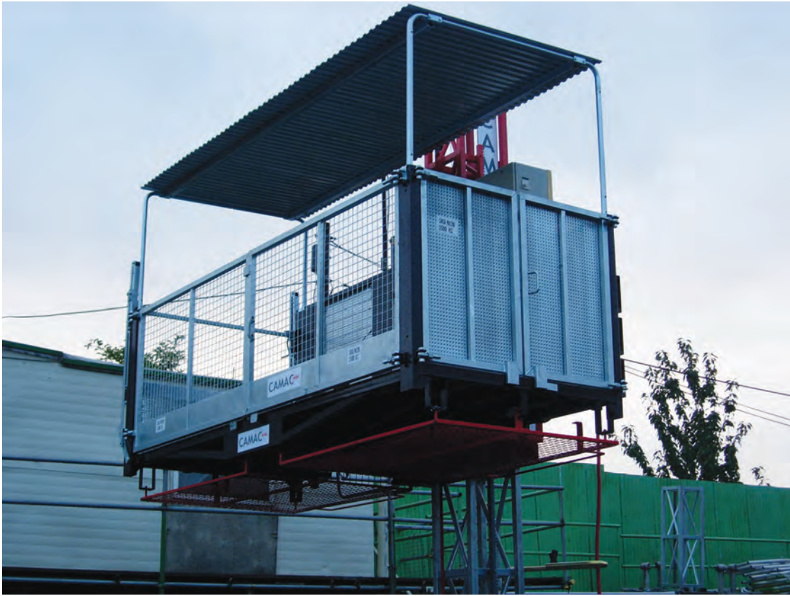
LEFT: Designed for lifting personnel and materials, Camac transport platforms have been growing in demand internationally. Here is one of the models, the ECP-1500, featuring a payload of up to 1,500 kg.
