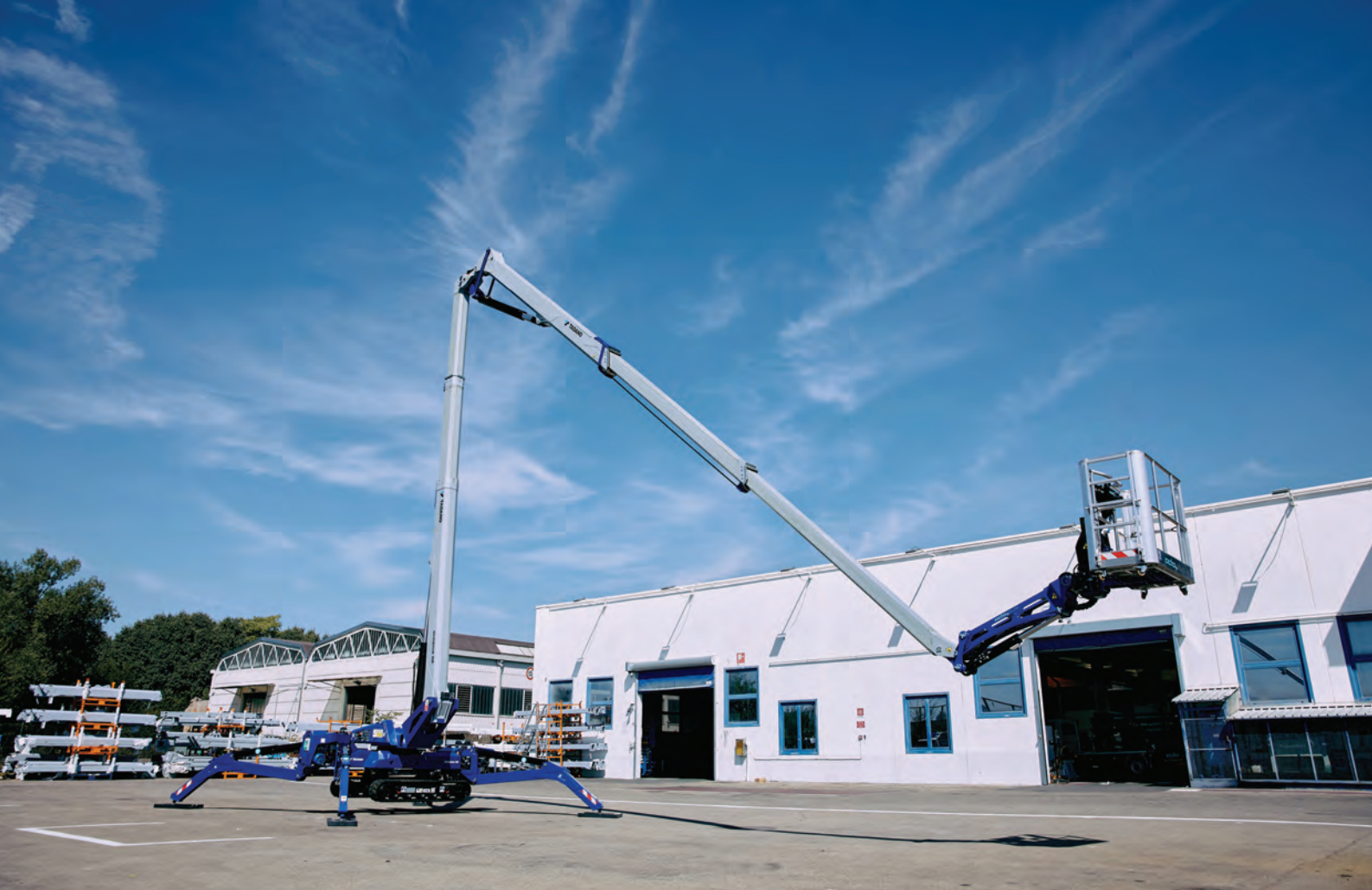
ABOVE AND BELOW: The Octopus 30 tracked platform has a maximum working height of 29.6 m.
