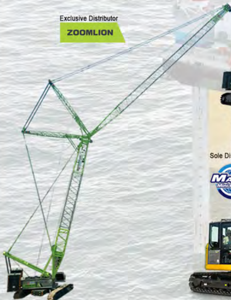
Crawler Crane with luffing jib
