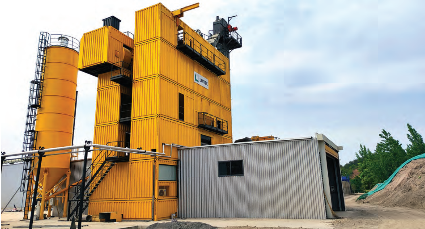
ABOVE AND BELOW: With a 240 t/hr capacity, the CSM3000 plant has already produced nearly 10,000 t of premium asphalt mix. Delivered as a complete turnkey project, the Lintec & Linnhoff team oversaw every stage of the process, from plant transportation and installation to commissioning and operator training.
