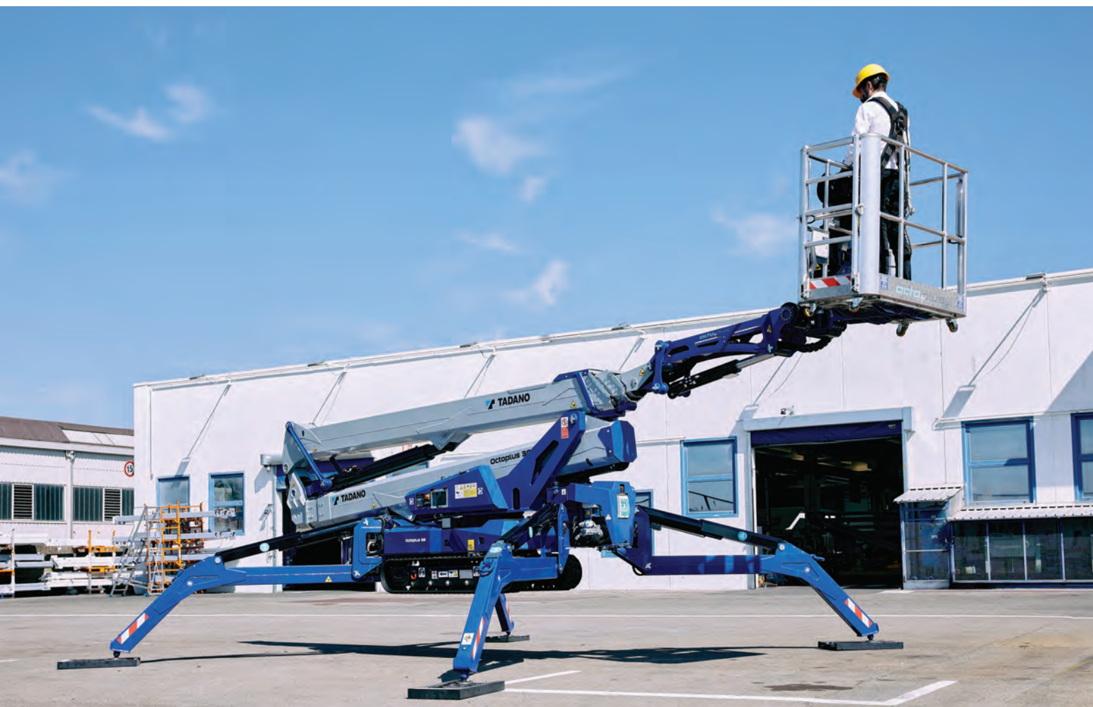
ABOVE AND BELOW: The Octopus 30 tracked platform has a maximum working height of 29.6 m.
