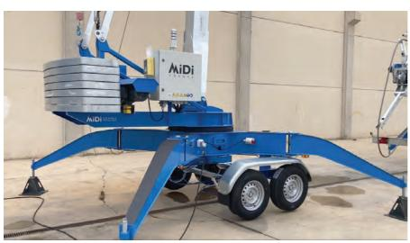
TOP AND ABOVE: SEAC had an opportunity to visit MiDi Cranes' facility in Zaragoza, Spain. The company manufactures compact, lightweight, road-towable self-erecting cranes weighing less than 3,500 kg. The machines are equipped with an electric motor.
