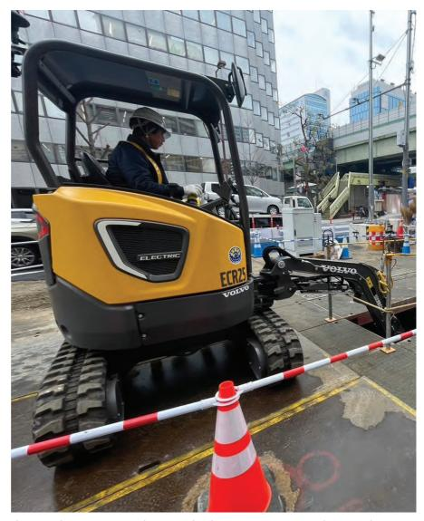
The ECR25 Electric excavator working on a railroad construction project in Osaka, Japan. The machine has a capacity of 2.6-2.8 t and a 20 kWh battery.
