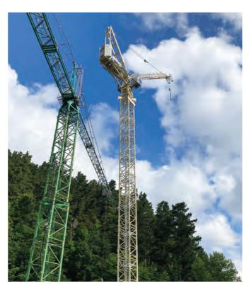
The new J638PA luffing crane (on the right) seen at Jaso's facility in Idiazabal, Spain. This model has a maximum reach of 65 m, with a maximum load capacity of 32 t and a maximum tip load of 7.2 t at its full reach.
